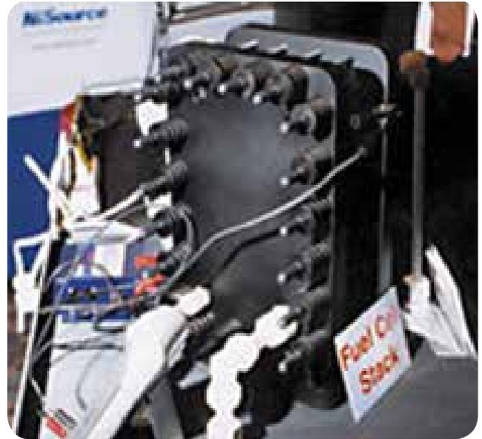
*A look at the basic fuel cell structure and connections (courtesy of NiSource Inc. subsidiary Energy USA).*
