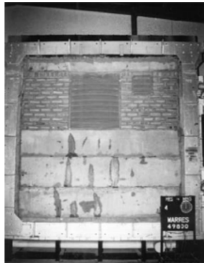
Warres 49800, Fire Resistance up to 4 hrs
