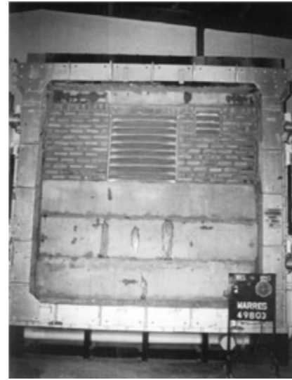
Warres 49800, Fire Resistance up to 2 hrs
