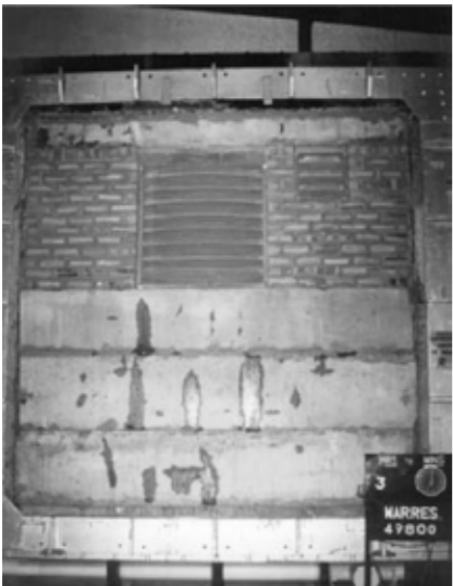
Warres 49800, Fire Resistance up to 3 hrs
